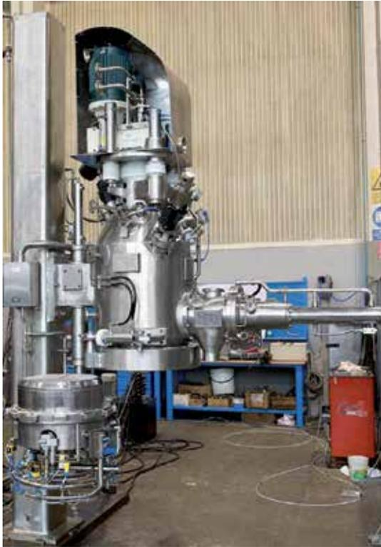
*Pressofiltro<sup>®</sup> agitated Nutsche filters / filter dryers in steam sterilizable design.*
