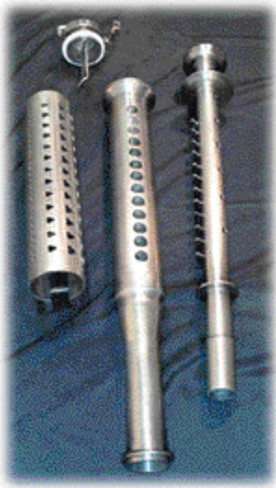
Easily disassemble the Nugget Former for cleaning.
