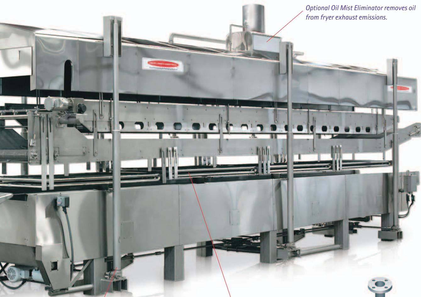
*Optional Oil Mist Eliminator removes oil from fryer exhaust emissions.*
