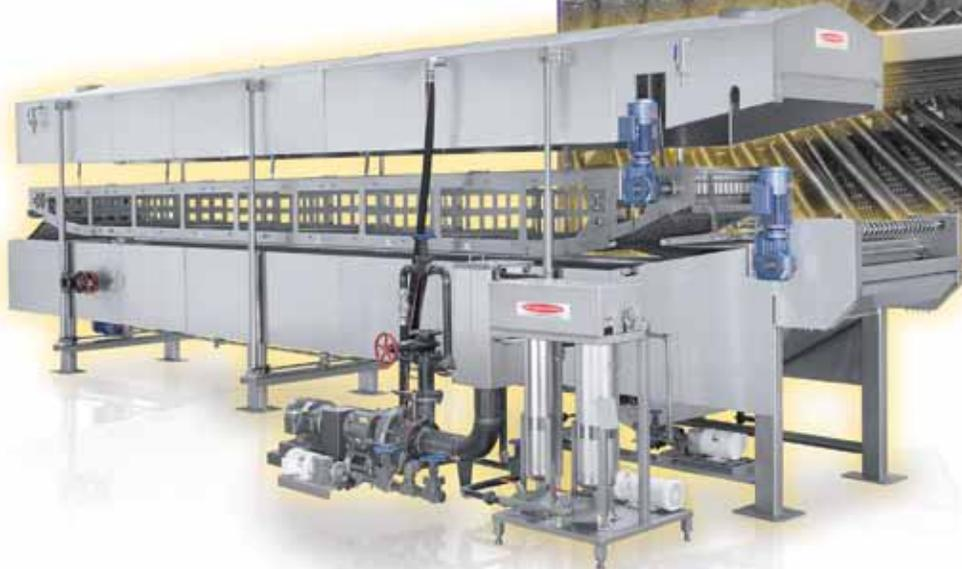
*Chip molds are easily removed. Shown with an optional Canister Filter, fryers are available with a variety of oil filters to suit your product.*
