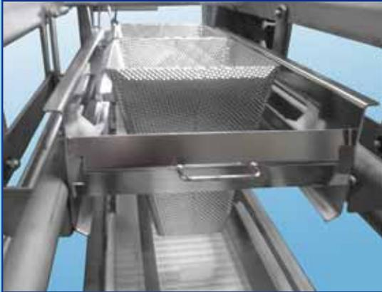
Our Dual Axis Funnel Follower transfers precisely weighed portions of dry, fresh or frozen products from your Ishida weigher into trays or cartons on a continuous motion horizontal conveyor.
