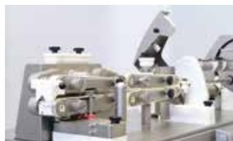
↑ Precise separating with 2-belt solution and sensor
