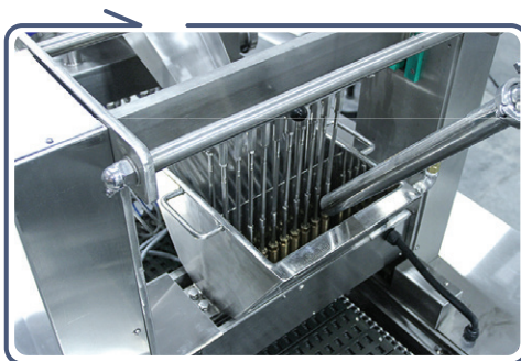
Dual Hoppers with Servo Drive Controlled Dosators (20). Automatic adjustment for easy fill volume changes. Fill volume range 1-15g.
