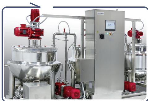
Sugar and glucose Dissolving Tank & Storage Tank with Control Panel .
