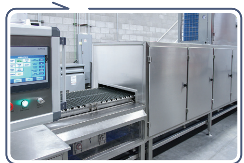
3 Level Cooling Tunnel with 15hp Chilling System & 0-20°C controls. Food grade final cooling belt.
