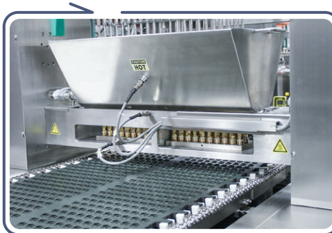
Dual Hoppers with Servo Drive Controlled Dosators (40). Automatic adjustment for easy fill volume changes. Fill volume range 1-5g.
