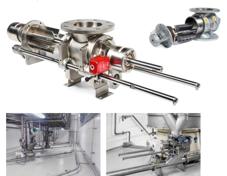
Lean or dilute phase conveying systems are the ideal solution for transferring bulk materials that do not require particle preservation and are not abrasive. Its advantage lies in the versatility of products that can be conveyed as well as in the space saving setup.
