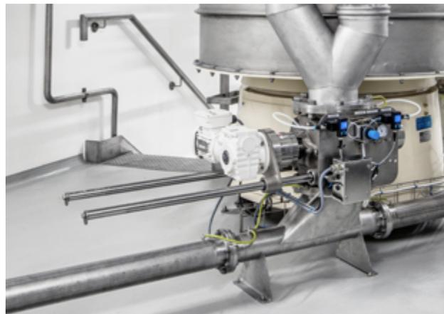
**Lean or dilute phase conveying systems are the ideal solution for transferring bulk materials that do not require particle preservation and are not abrasive. Its advantage lies in the versatility of products that can be conveyed as well as in the space saving setup.**
