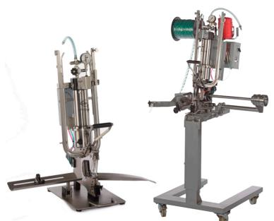
service-friendliness. The valves are installed on a service-friendly, "easy-to-change" pullout bar. Quick and easy replacement of worn valves means short down-times and increased efficiency. The open design in the filler and closing areas makes easy access to the work area an outstanding feature. Thanks to the well thought out design, service work can be carried out quickly and easily.
