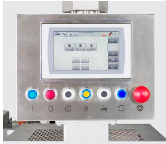
**The controls and product adjustments are managed by the Human Machine Interface (HMI).**
