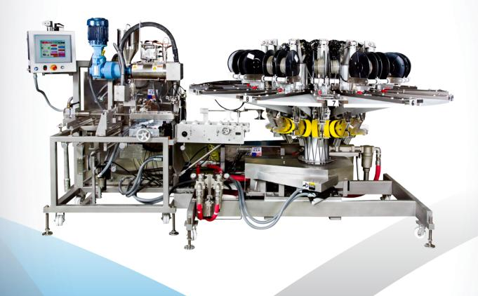
Automated heat-seal and clipping of pumpable products in flexible packaging
