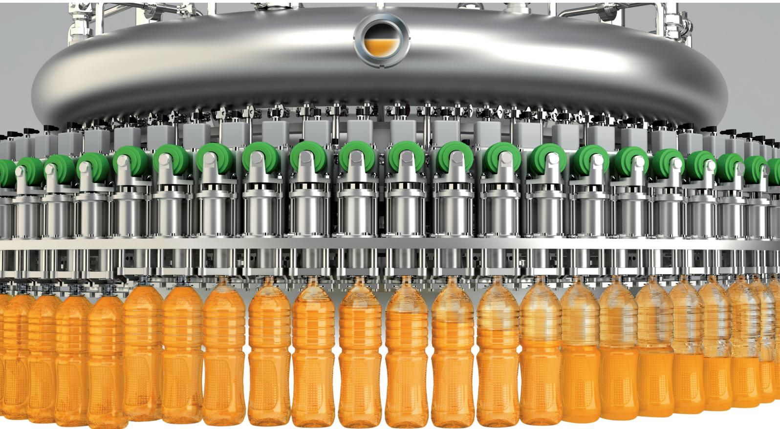
The present tendency of CSD products is to emerge as a healthier product, thereby reducing or eliminating the use of preservatives. In order to comply with the need of a cleaner filling process within a hygienic environment, GEA Procomac introduces the new range of counterpressure fillers Fillstar LXi.
