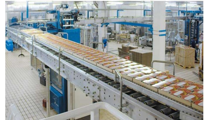
GEA’s product range includes the most diverse solutions suitable for handling cartons and crates of very different sizes and consistencies.
