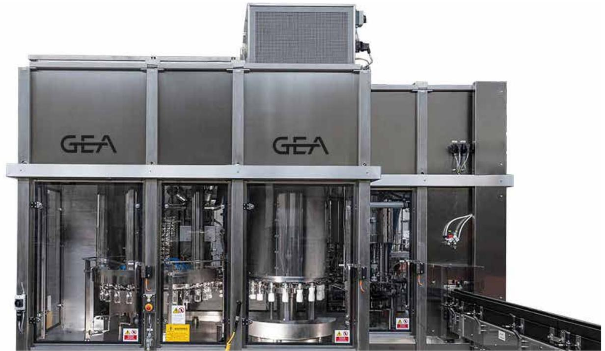
The bottle decontamination treatment is performed in a hygienic cabin where a clean and protected environment is maintained thanks to a top-down laminar flow of sterile air. On the same carousel, both H<sub>2</sub>O<sub>2</sub>-based solution injection and subsequent activation with warm air are carried out.
