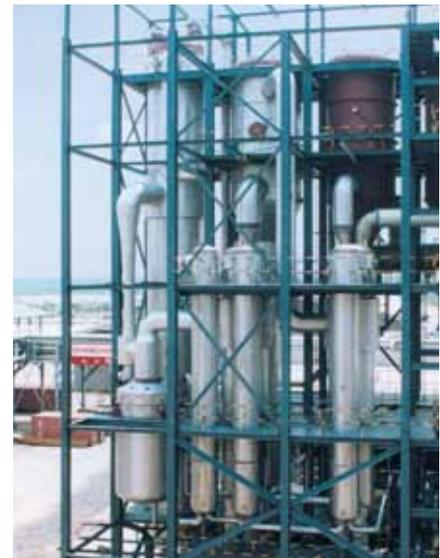
*Three-effect falling film forced circulation evaporation plant with thermal vapour recompressor for waste water from monosodium glutamate production. Evaporation rate: 50 t/h*
