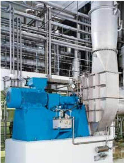
Mechanical vapour recompressor (centrifugal fan) of a single-effect falling film evaporation plant in food production
