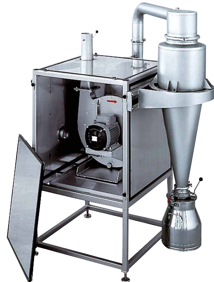
For reducing noise from fans, a noise attenuator is an effective solution.
