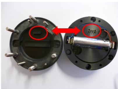
8. Ensure that the plug contacts are in the correct position when closing the battery compartment!
