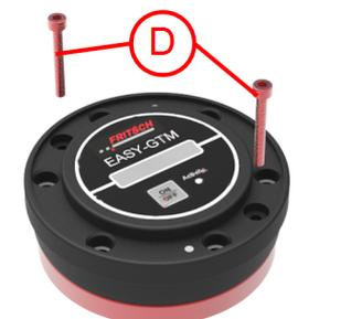
5. → Undo the two screws (D) of the battery compartment using a hexagon offset screwdriver, size 2.5 mm (7).
