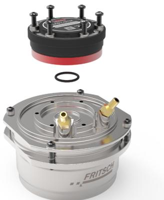
3. → Lift the measuring/transmission unit (9) off of the lid (11).
