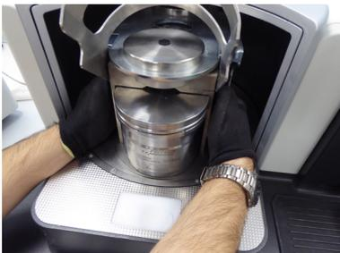
Once the shield is opened and the grinding bowl has been released completely, you can press it out from behind as shown.
