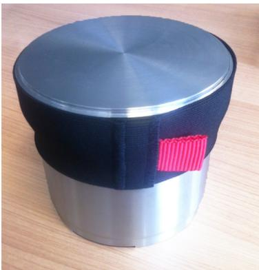
1. → Once the grinding balls are placed in the bowl with the sample on top, put the lid on the grinding bowl.
