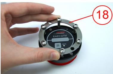
Remove the lock ring (18), incl. screws, from the measuring/transmission unit and remove all soiling.
