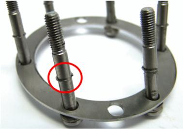
The screws are equipped with a circlip to prevent them from falling out of the lock ring (18). Ensure that the circlips are sitting correctly! (See illustration!)
