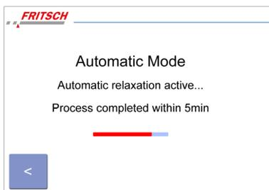
A screen with a progress bar is displayed during automatic unclamping. This indicates approximately how much longer the unclamping process will take.
