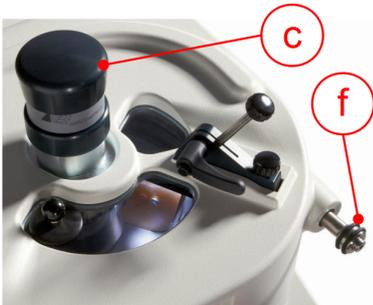
2. ➤ Insert the pestle into the latch bearing in the lid (see Chapter ➔ Chapter 6.3.2 'Installing/removing the pestle' on page 22)
