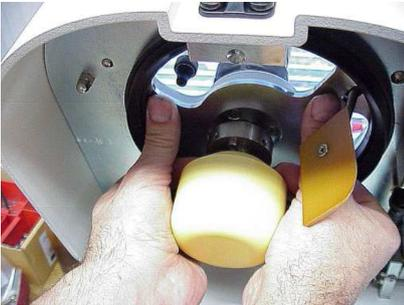
The pestle is held in place with a catch holder and can be easily removed without tools.
