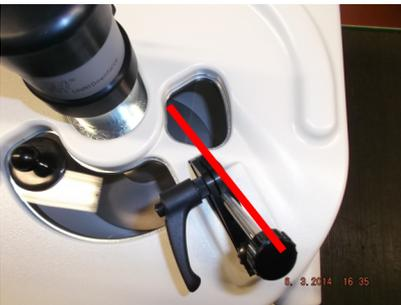
5. ➤ Tilt the guide rod while turning the scraper to the left to align it with the guide rod.
