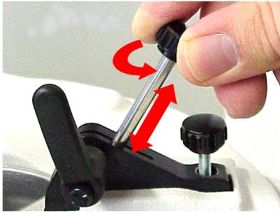
4. ➤ Move the scraper against the wall and onto the bottom of the mortar by turning it to the left.
