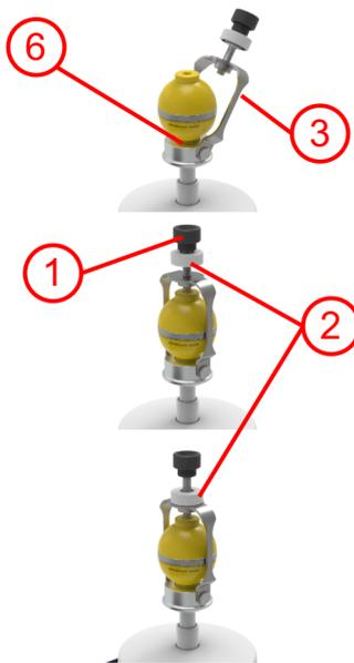
1. ➤ Before clamping, check the rubber disk (6) in the base of the grinding bowl holder for any damage.
