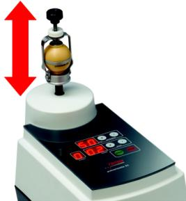
The rapid vertical acceleration of the grinding bowl causes the grinding balls in the bowl to vibrate. Comminution occurs when the balls of grinding stock hit the walls of the bowl and each other. Due to the almost spherical grinding chamber the balls are not limited to vertical movement, and very efficient comminution is achieved.
