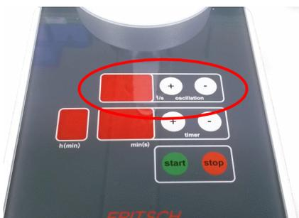
The vibration frequency can be set as 15-50 Hz (strokes per second) in 1 Hz steps using the +/- buttons (oscillation). The mill generates natural oscillation of higher or lower intensity depending on the stroke frequency. The set oscillation frequency is controlled by the microprocessor and thus guarantees reproducible grinding.
