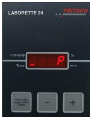
You can switch between the feed rate and timer function settings with the Intensity/Time key. Press the Intensity/Time key until the light bar indicates the word Time.
