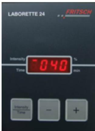
You can switch between the feed rate and timer function settings with the Intensity/Time key. Press the Intensity/Time key repeatedly until the light bar indicates the word Intensity.
