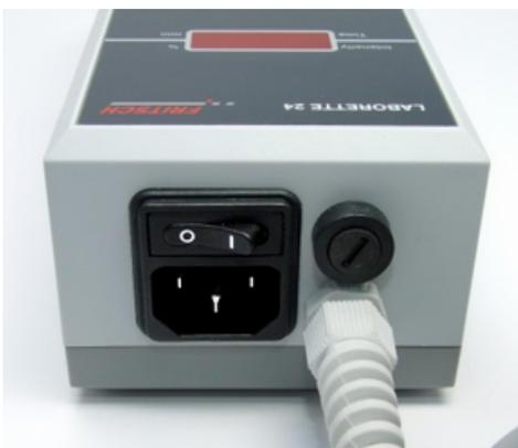
Actuate the main switch on the rear of the device.
