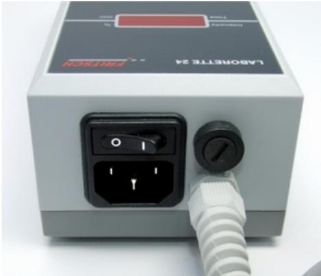
The control box contains a mains connection socket with mains switch, a device connection cable with plug and a T1.25A device fuse (5x20).
