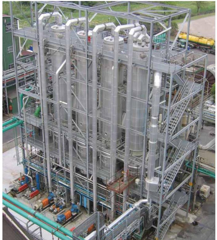
installation costs are lower. The replacement of required steam with recycled vapor results in lower operating costs making this a viable choice in many applications. This is a very attractive option for larger evaporation rates.
