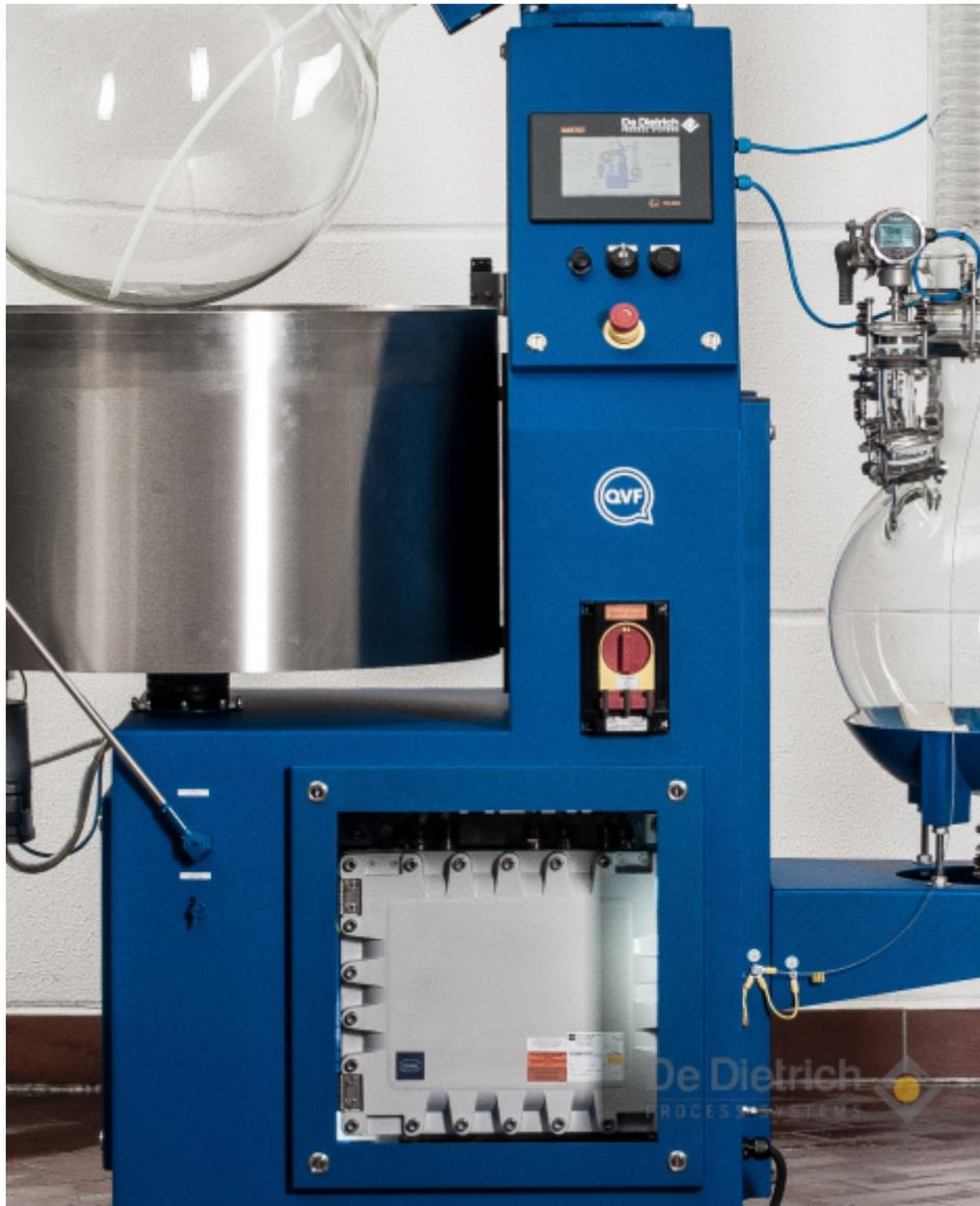
QVF® ROTADEST with visible EX-housing for demonstration
