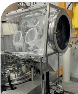
This solution allows you to charge powders manually and directly from a drum to your reactor in total safety. The station can be designed as per your environment all constraints and will be perfectly adapted to your needs. The DIT® system is integrated to reach optimal performance.
