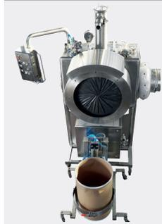
The docking of drums for powder transfer could represent a challenging yet necessary operation while developing most production processes, especially when high containment is a must.
