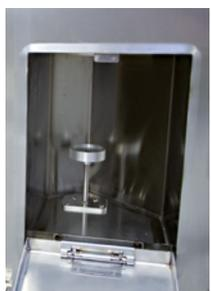
The machine is fitted with a syringe unloading system with ventilated duct between chamber and transport container. The system allows you to unload the dispensed syringe directly into the specific shielded container.
