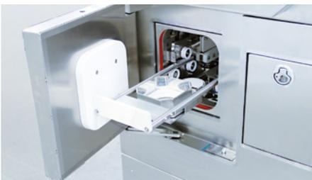
The prechamber is equipped with a sliding tray and a pneumatic lifting device to introduce or extract materials from the work surface.
