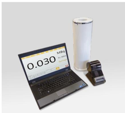
The IBC Dose Calibrator is a completely digital dose calibrator. The ionisation chamber is connected directly to a PC with Windows. Like all Comecer dose calibrators, each model is used in combination with a completely digital VIK-202 model ionisation chamber.
