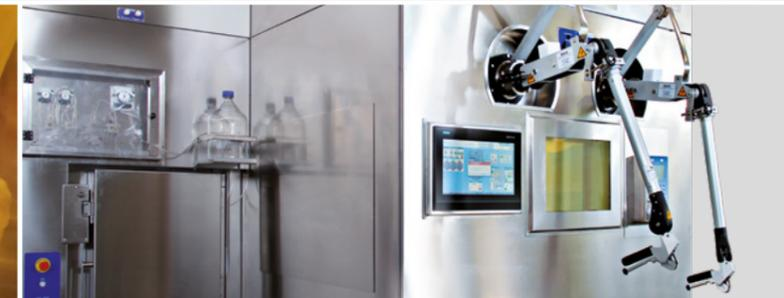
Production plant consisting of two high-shielding hot cells in which it is possible to perform fractionation, calibration and preparation operations for shipment of <sup>99m</sup>Mo bulk.
