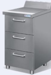
This drawer safe is used for the combined storage of radiopharmaceuticals and Tc-99m generators. The safe is also perfectly suited for the storage of PET waste. The drawers are shielded with lead and are lined on the inside with stainless steel. All drawers share a common lock. The outside of the safe is made stainless steel with Scotch-Brite™ surface finish.
