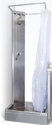
Decontamination Shower with discharge into the drainage system. Basement stainless steel shower tray with raised edge to contain liquids. Column equipped with mixer for the manual regulation of the water flow and upper spray nozzle. Upper spray nozzle, PVC tent. Liquid collecting polyethylene container for decay, placed in the right compartment underneath the shower, and sensor that stops automatically the water flow once the maximum level is reached (only for SC model).
