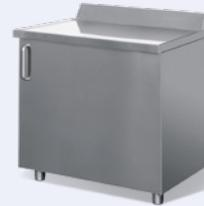
The model KK-102 consists of a stainless steel worktop with an integrated shielded laboratory refrigerator with a capacity of 120 litre and a temperature range from 2° to 20° C (digital read-out) with an acoustic alarm in case of deviation. The refrigerator has 2 interior racks allowing different heights for storage. The interior of the storage safe is lined with stainless steel. The exterior of the storage is made of stainless steel with Scotch-Brite™ surface finish.
