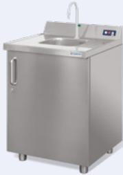
Stainless steel sink with hinged door. Worktop with raised border for holding the liquid and no sharp edges to allow the perfect removal of any radioactive residuals. Sealed lower containment compartment to prevent the leakage of liquids. Hinged front door with a key lock. Swan neck faucet for the regulation of water flow. Water flow command via photoelectric cell.
