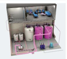
7) **Overflow unit:** it allows the collection of sewage that could come out of the tanks (for component breakage or level control failure) and transfer to sorting unit.
