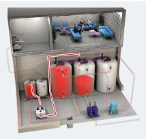
*4)* Clarified water sorting at decay tanks: this units allows collection and decay of radioactive liquid coming from the sorting unit.
