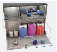
6) **Discharge unit:** after sample measurement, if the activity and concentration levels are below preset values, the examined tank can be discharged by pressing the appropriate button on the control panel.
