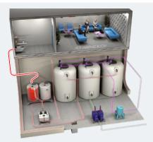
2) **Purification unit:** treatment of waste coming from the department with separation of solid part and subsequent anaerobic biodegradation of the latter.
