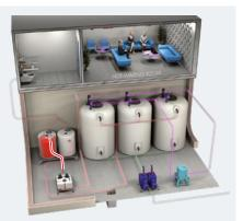
*3)* **Post imhoff lifting unit:** this unit is a compact and sealed tank with two electric submersible pumps and a system that prevents blockage of the impeller in the presence of large quantities of materials.
