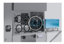
**Connect and use**: the incubator is aseptically connected by an RTP to the isolator and opened in a grade A environment.
