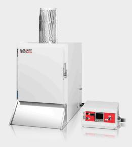
Clean room oven CR130 with oxygen sensor for high humidity atmosphere applications according customer specifications
