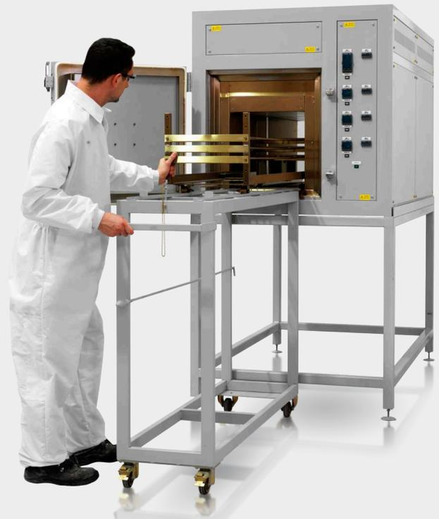
Custom designed GPC General purpose chamber furnace to fit into a clean room wall (Ref. no. 300904)
