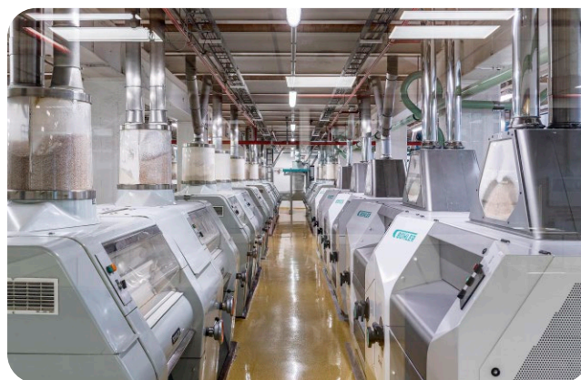
Old/new comparison: The (still) old roller mills of the A mill on the right, the new Diorit MDDY of the B mill on the left
