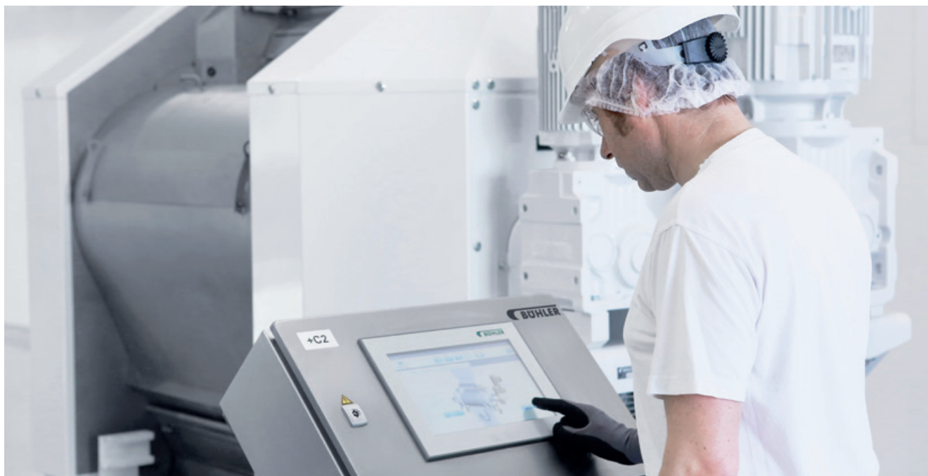
The EasyFlake machine control system with touch screen interface makes configuration of production parameters easy and safe
