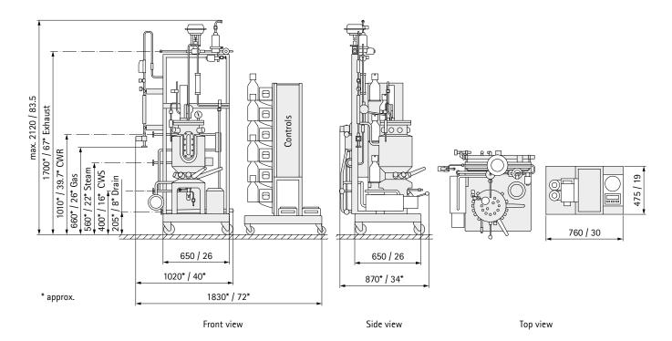
Dimensions are given in mm and inch and represent maximal values. Depending on fermentor configuration dimensions can be also smaller. White parts of drawing represent variable areas according to selected options.
