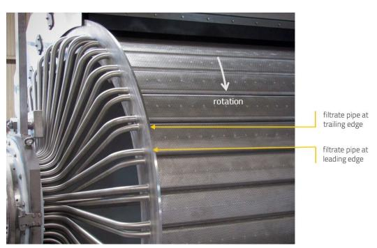
YouTube has been restricted due to privacy settings Filtrate pipes at leading and trailing edge of filter cells
