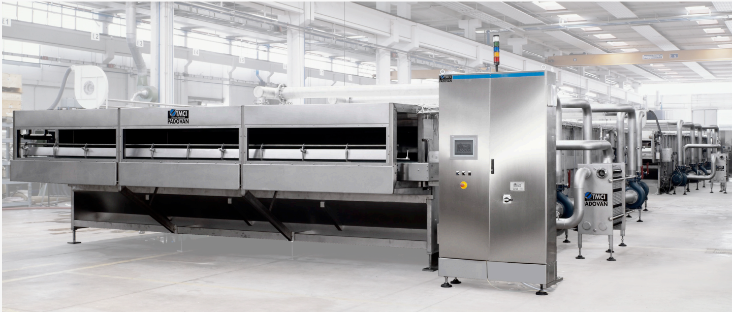
Twin cooling tunnels
