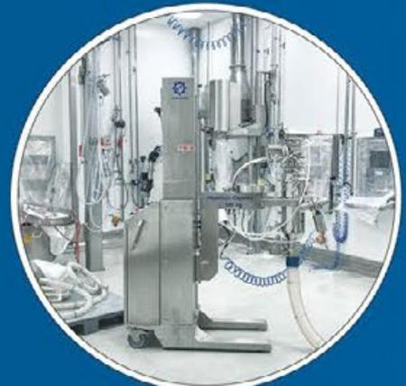
Automatic Mobile Lifting Column for Vacuum Conveyor
