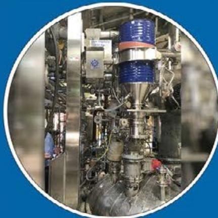
Fixed Automatic Drum Lifter for Reactor Loading
