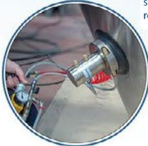
*Bottom Valve with clamp connection*
