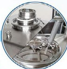
*Lid with the installation filter pre-arrangement*
