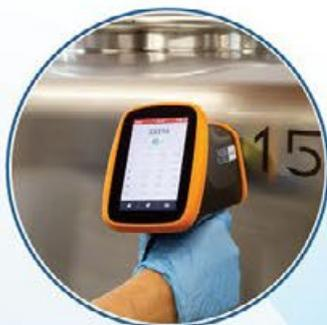
*All produced machinery undergoes control procedures including the quality verification of the construction materials (e. g. stainless steel 304, 316, 316L, etc.) using XRF Alloy Analyzer (Gun)*
