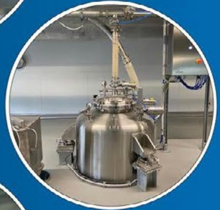
VTS Hoppervac for powder dosing system to charge a mixer
