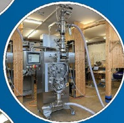
Vacuum Conveyor to load a Roller Compactor
