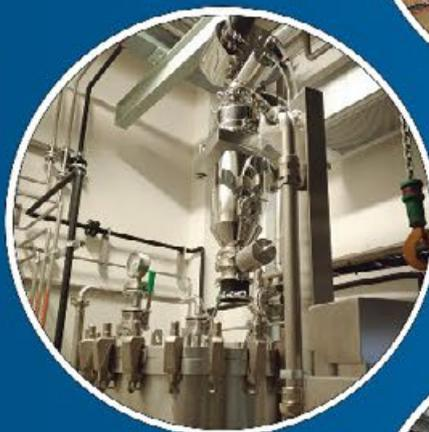
Vacuum Conveyor on a Lifter for loading a plate Filter
