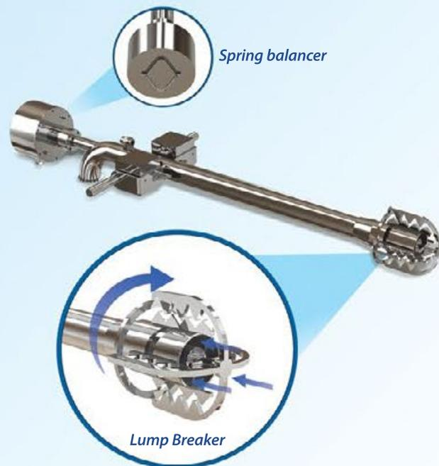
AGIERRE's **Lump Breaker Lance** is an enhanced Suction Lance configuration specifically designed to suck humid powders prone to clumping into large pieces that would otherwise get stuck in the standard version. The equipment is manufactured from AISI 316L stainless steel with a mirror-polished finish on internal and external surfaces.
