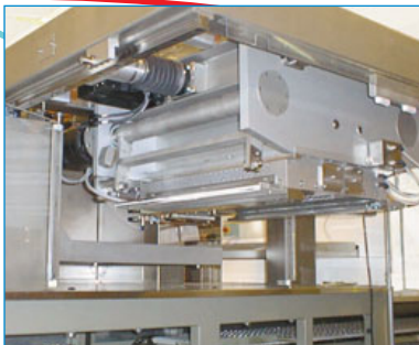
In-line depositor in off-line position for cleaning and maintenance.
