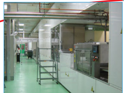
Shell section showing EP2 in-line depositor for almost any kind of masses.
