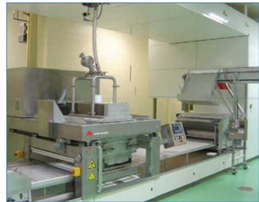
Depositor type ET in-line for caramel centre depositing.
