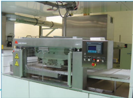
Shell centre section showing SE12 in-line depositor for depositing centre fillings with or without ingredients.
