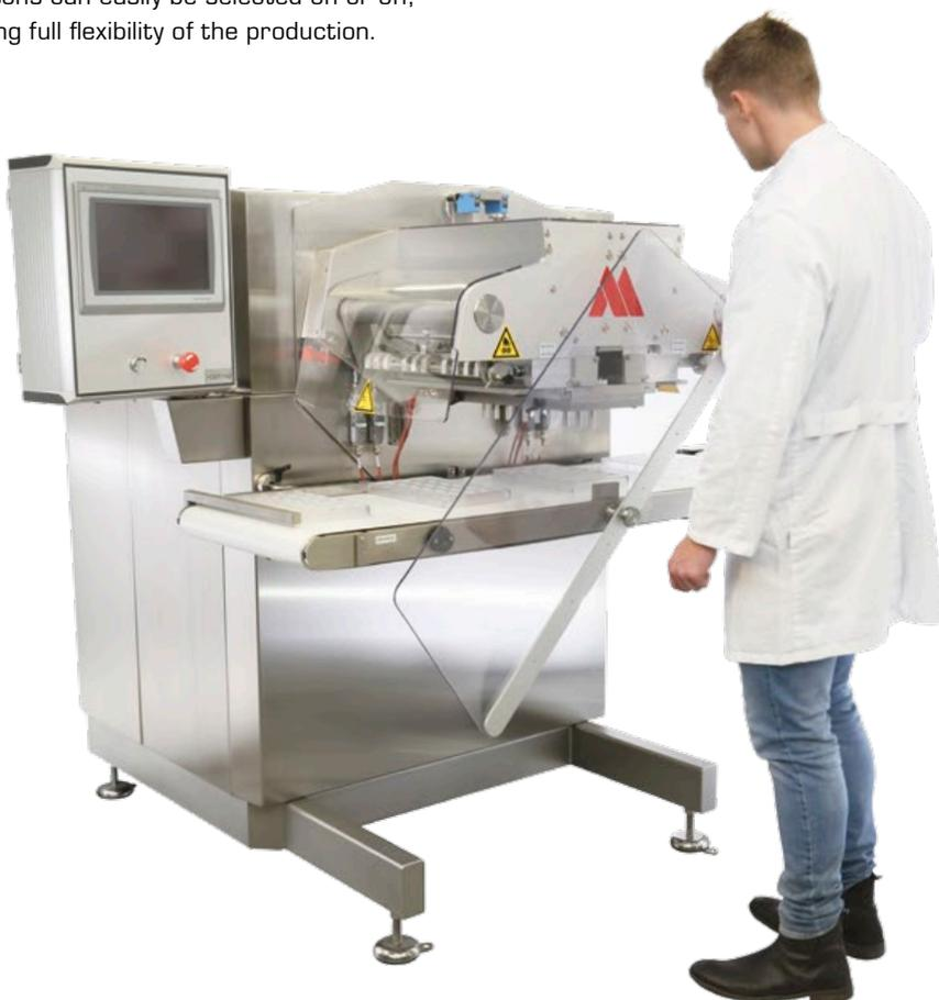
The Nilshot works with many types of moulds, and the flexibility of the pistons allows full control of the production. The turnable safety screen insures safety for the operator and allows for easy access, when it is in open position.
