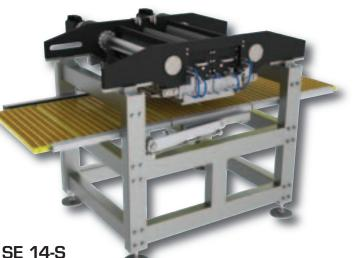
Detachable hopper and depositing parts are options which much enhances cleaning and shift of tools at production shift or when required.
