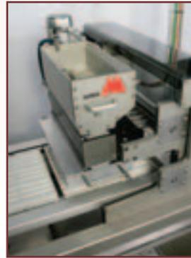
*SF depositor version - with servo driven piston movement, which ensures high precision depositing*
