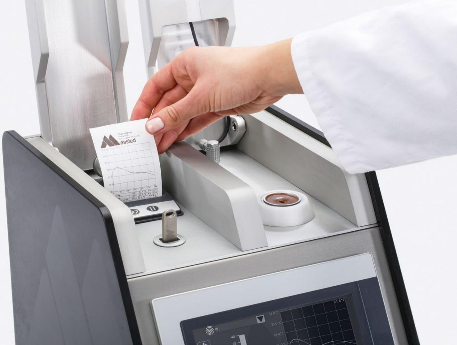
*Chocometer+ calculates the CTU (Chocolate Temper Unit) and the slope. It also computes and displays the Temper Index (TI).*
