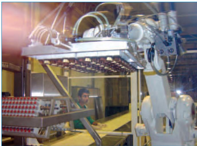
All the differently coloured and shaped articles are moulded in the same pressing operation and transferred by the robot in the same order directly from the moulds to the box.
