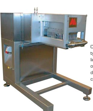
Customized servo-electrical depositor, type ESA, for a high capacity moulding line and designed for accurate dosing of aerated masses. Volumetric piston displacement under pressure in a closed manifold.
