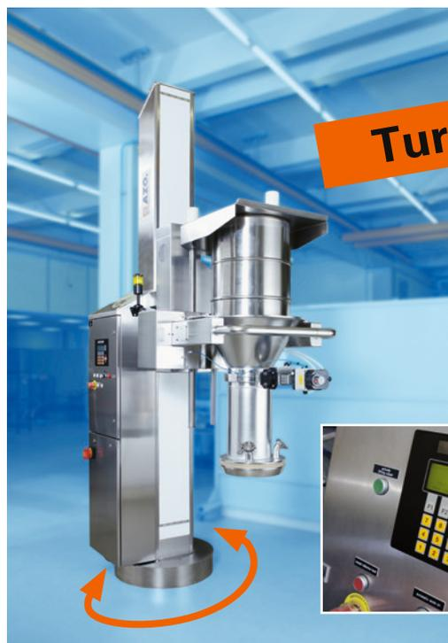
The Lifting column can be turned manually (up to a load of 400 kg) or by means of an electric drive.
