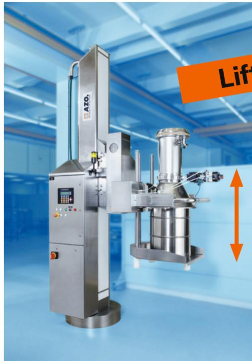
A freely programmable controller lifts modules or docked drums accurate to the millimetre.
