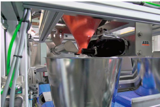
The products are dosed into the target container with an accuracy of up to  $\pm 2$  g (depending on the raw material and flow behavior) via the AZO®eDos dosing system. Advantages: simple geometry, easy to clean, hygienic, easy to dismantle
