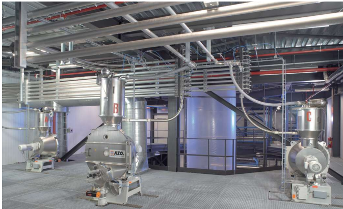
AZO®MIXOMAT scale for loading foil blower extruders
