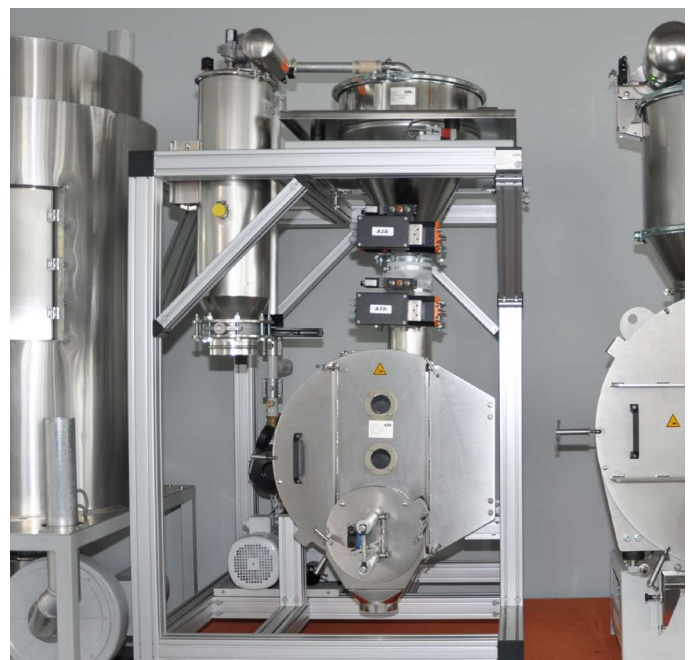
AZO®MIXOMAT conveying scale directly over extruder, masterbatch is weighed separately, additive in powder form is negatively weighed into the masterbatch scale using AZODOS®
