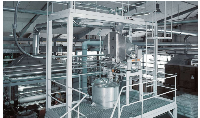
AZO®MIXOMAT scale above processing machine
